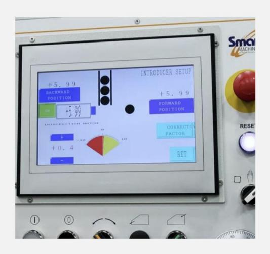
Auto-Setup – dedicated software that allows for job storage of over 2000 programs and the technology for quick setup of several functions such as Die Match, Injector position, and vertical position of rails and vibe bowl.
