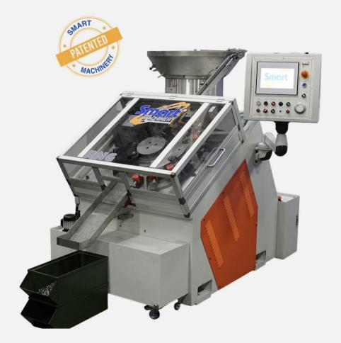
RNG Machines are compact, fast, flexible, and can handle small or large lots of various sized product ranging from M6 up to M24. Machines are equipped with patented Direct Drive gear-less technology, high precision Linear Motors, Die matching adjustment, and easy-to-use Auto set-up for quick, repeatable set-up.
