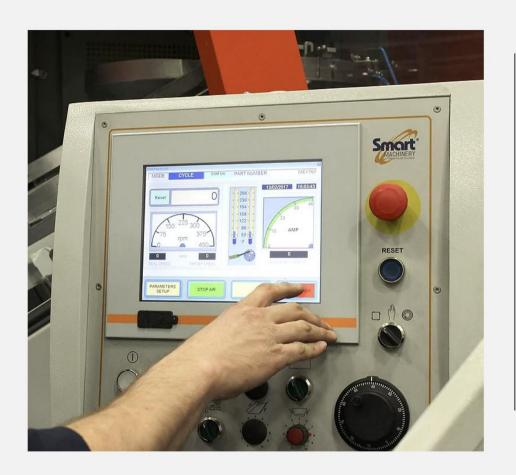
Auto-Setup – dedicated software that allows for job storage of over 2000 programs and the technology for quick setup of several functions such as Die Match, Injector position, and vertical position of rails and vibe bowl.
